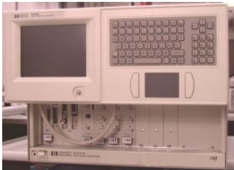
Figure 12 Option 001 connected to a standard HP E4840A small mainframe
