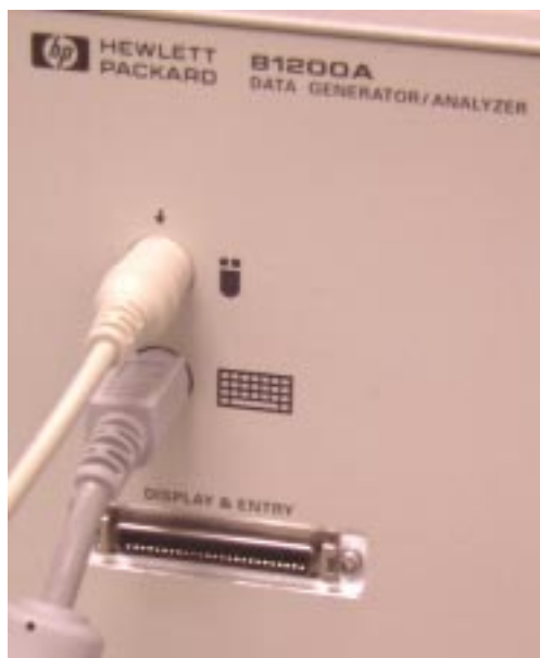
Mouse and Keyboard to connect on the Front Panel of the HP E4840A Small Mainframe
